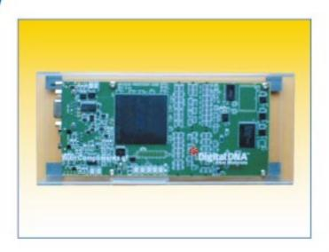
The MPC8260 Processor Card functions as a generic MPC8260 resource board, provides a flexible environment for developers implementing MPC8260-based networking application. It is a self contained system with MPC8260 and some peripherals assembled on a small PCB, included system memory and boot Flash on its 60X PowerPC bus and system memory on local bus.
