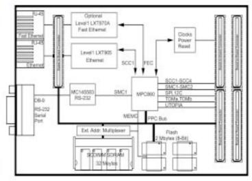
The MPC860 Processor Card functions as a generic MPC860 resource board, provides a flexible environment for developers implementing MPC860-based networking application. It is a self contained system with MPC860 and some peripherals assembled on a small PCB, included system memory and boot Flash on its local PowerPC bus.
